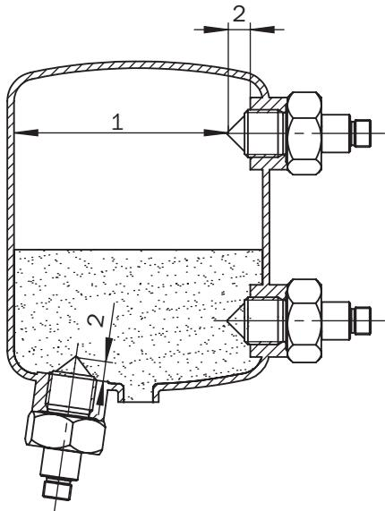
The apex should protrude into the container
