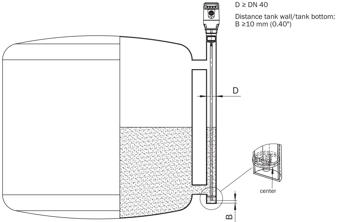
Instruction for installation Installation in a metal tank
