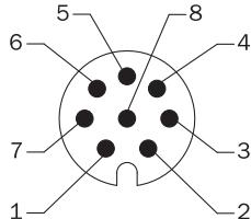
view of M12 male device connector on cable / housing
