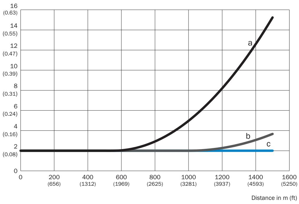
Repeatability DL1000 for various reflector types, with 16 ms measurement cycle time
