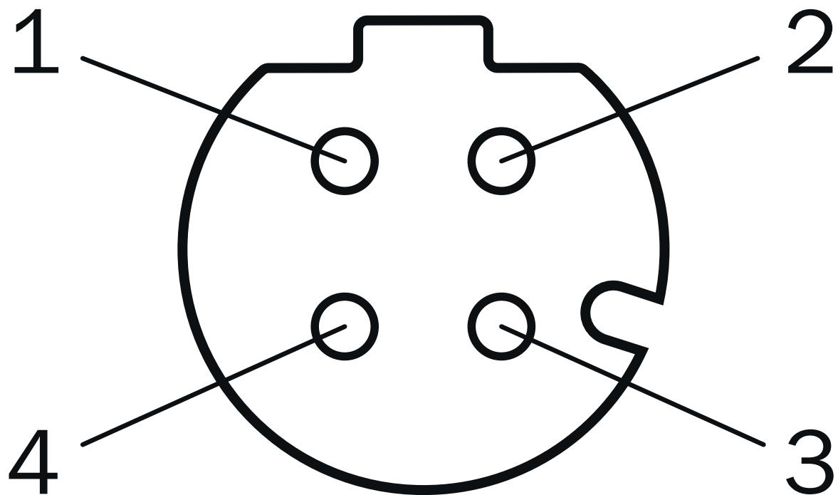
M12 female connector, 4-pin, D-coded
