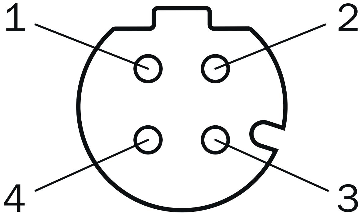
M12 female connector, 4-pin, D-coded
