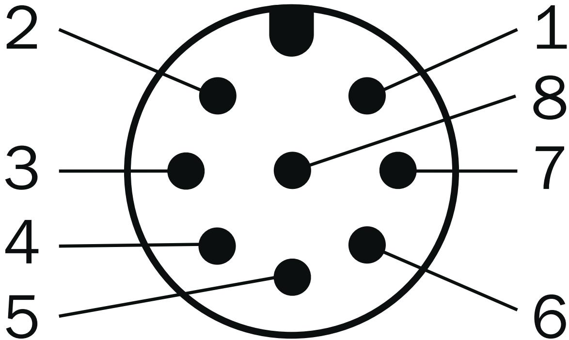
Connector M12, 8-pin, A-coded
