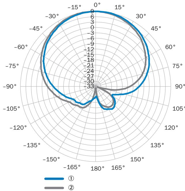
measured antenna gain in dBi at 868.5 MHz, RHCP (right-hand circularly polarized)
