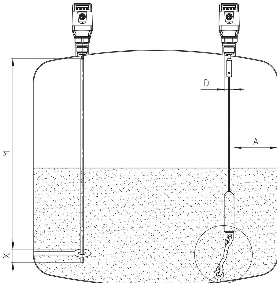
**Mono rod probe mounted in metal tank**
