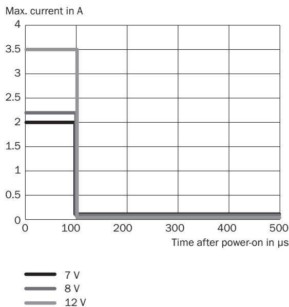
This diagram shows the switch-on current
