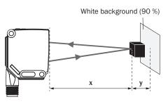
Black object (6 % remission) Set sensing range  $x=80\ mm$  Needed minimum distance to white background  $y=0.5\ mm$
