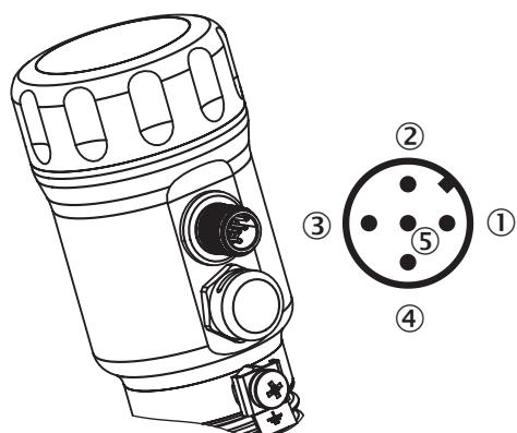
① L<sup>+</sup>: Supply voltage, brown② Q<sub>A</sub>: Analog current/voltage output, white
