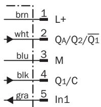
**PIN assignment Connector M12, 5-pin, A-coded**
