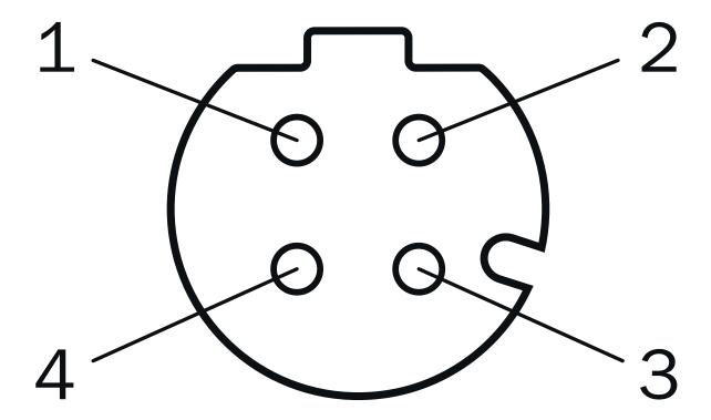
M12 female connector, 4-pin, D-coded
