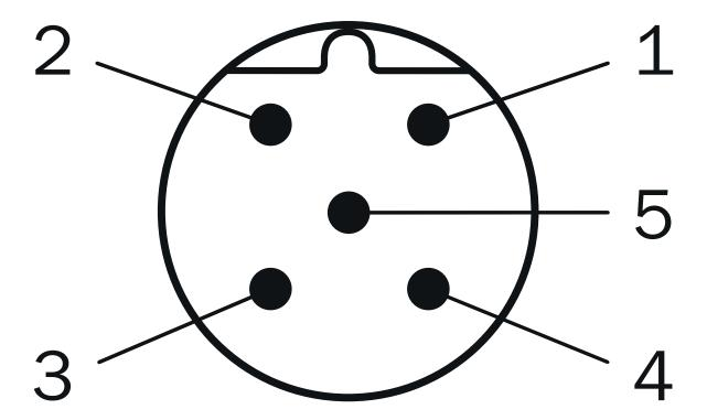
Connector M12, 5-pin, B-coded, BUS IN
