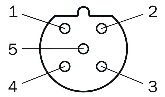
Female connector M12, 5-pin, B-coded
