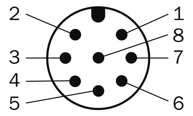
Connector M12, 8-pin, A-coded
