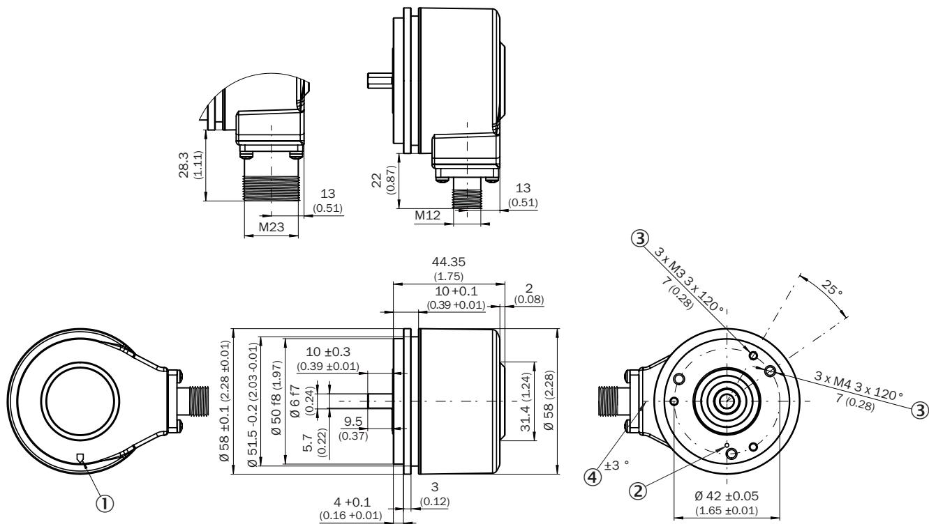
Attachment specifications Mounting requirements for small servo clamp
