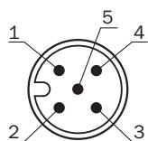
Connection diagram UM18-21xxxAxxx\_Bxxx, male connector M12, 5-pin
