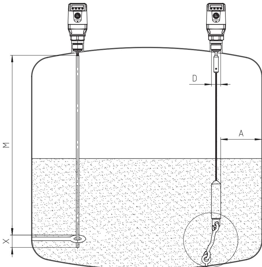
**Mono rod probe mounted in metal tank**
