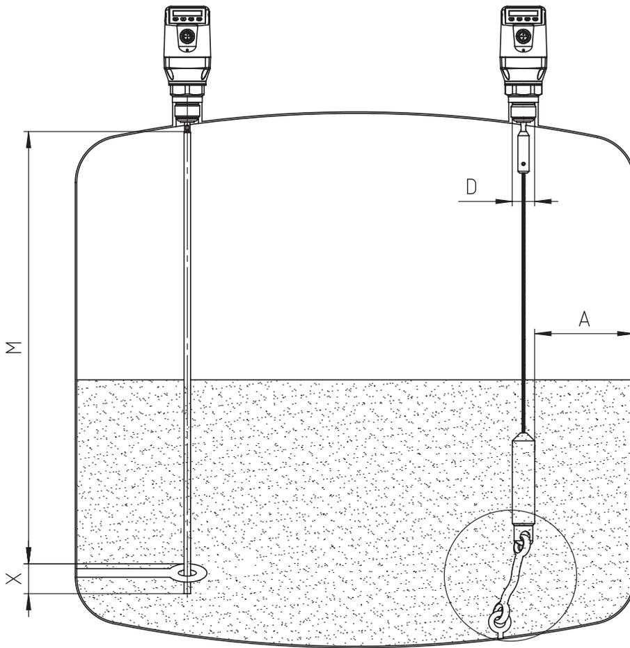
**Mono rod probe mounted in metal tank**
