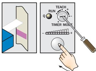
If yellow LED illuminates, turn rotary switch to "-" position and press and hold teach-in button until yellow light just goes out (green LEDs go out on the bar display).
