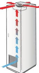
A roof ventilation supports the flow of warm air from bottom to top and avoids heat accumulation in the upper area. Here, the DE 400 roof vent (without fan) ensures natural ventilation. It is used when there are no special requirements for the degree of protection. A robust sheet-steel hood with stepped rim prevents water from entering. The filter mat is replaced from the inside.
