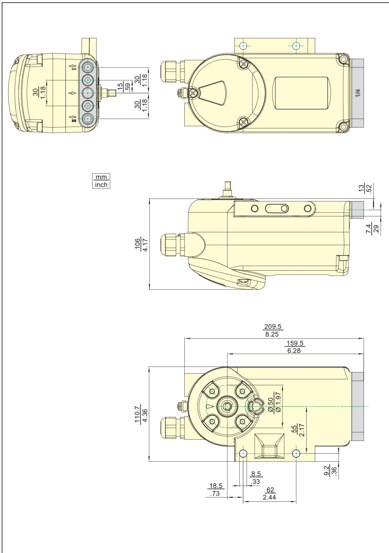
**DIMENSIONS with gauges and manifold**
